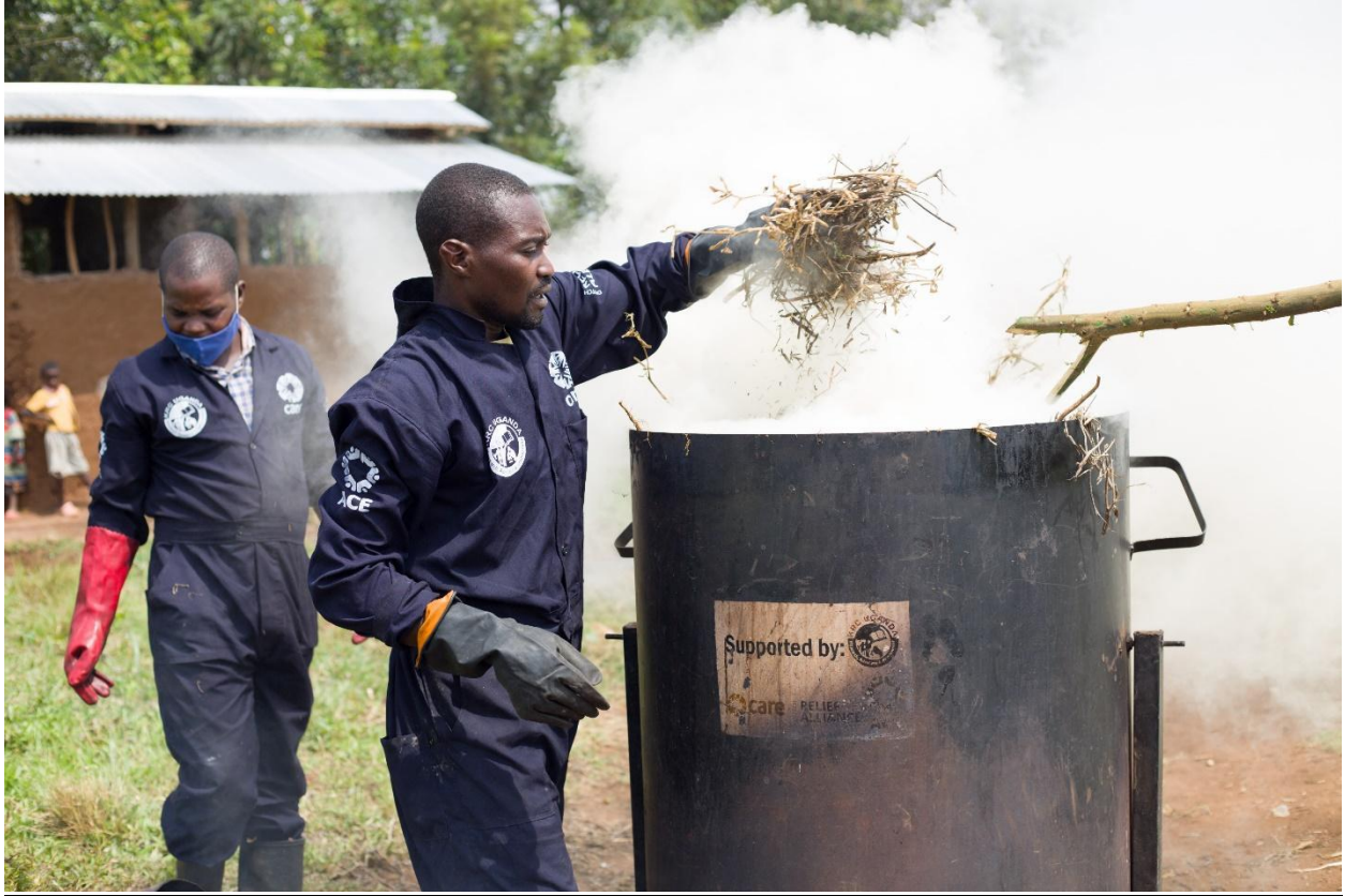
Photo 7: Tuwungane Nguvu members here preparing char that will be used to make the briquettes.
